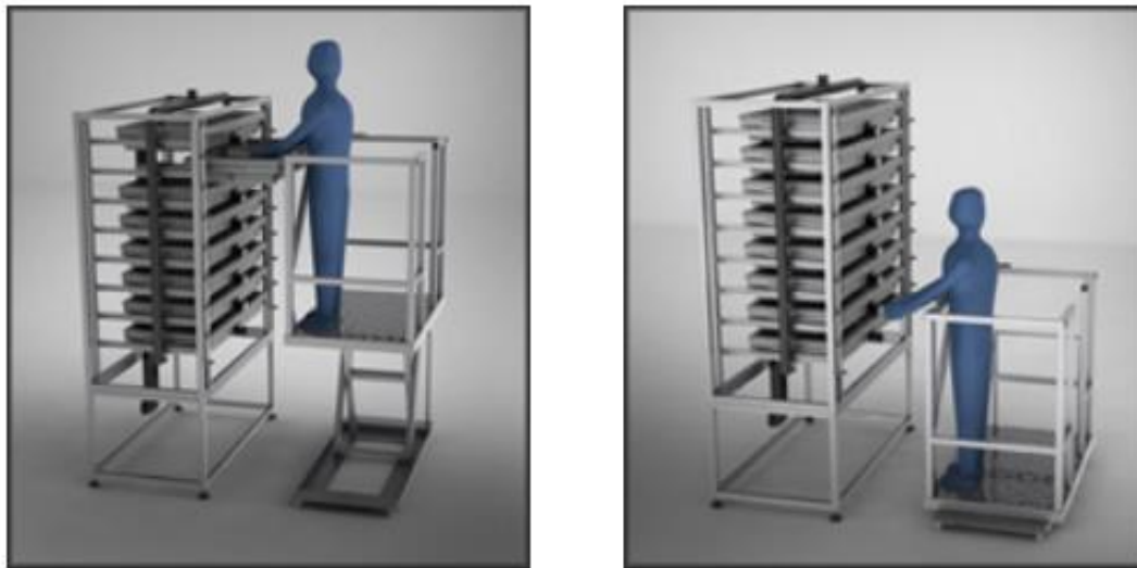
Figure 7. CompHatch hatching system illustration demonstrating the inclusion of a work lift
